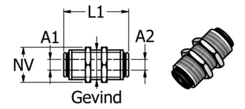
Ext. hose diameter A1 = 14 Ext. hose diameter A2 = 14 L1 = 45.9 NV = 27 Thread = M24x1
